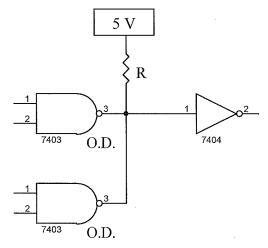
(a) For the case of BOTH inputs of BOTH gates driven LOW: If the off-state leakage current of each of the 74x03 open-drain NAND gate outputs is  $+5~\mu A$ , and the  $I_{IH}$  required by the 74x04 inverter is  $+490~\mu A$ , determine the maximum value of R that will produce a  $V_{IH}$  of at least 4.5 volts at the 74x04 input.
