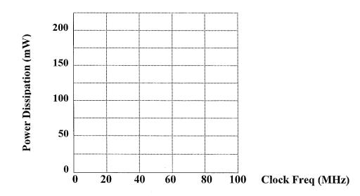
Assume a CMOS microprocessor dissipates 100 milliwatts of power when operated at a clock frequency of 100 MHz with a supply voltage of 5 V. If the frequency of operation is reduced from 100 MHz to 40 MHz (and the supply voltage remains 5 V), the power dissipation will be reduced to:
