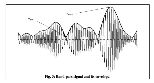
2. In Figure 3,  $e_{\text{max}}$  and  $e_{\text{min}}$  are the maximum and minimum of the envelope of s(t). Assume that  $\max(m(t)) = \max(-m(t))$  and show that the modulation index is:
