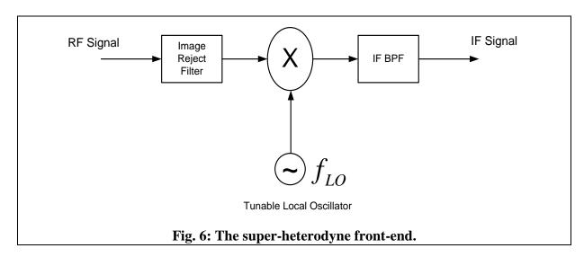
A simple super-heterodyne front-end consists of:
