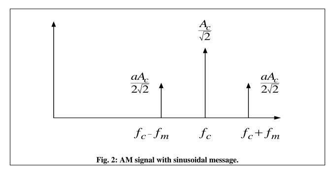
If the message is a tone, the AM signal will be as shown in Figure 2. (RMS values are shown in Figure 2; hence the factor of  $\sqrt{2}$ .) Furthermore, the spectrum analyzer provides no phase information (it is a scalar radio receiver); it displays the one-sided spectrum. On the other hand, a 'Vector Signal Analyzer' is capable of processing phase information and is frequently used to analyze digitally modulated signals.
