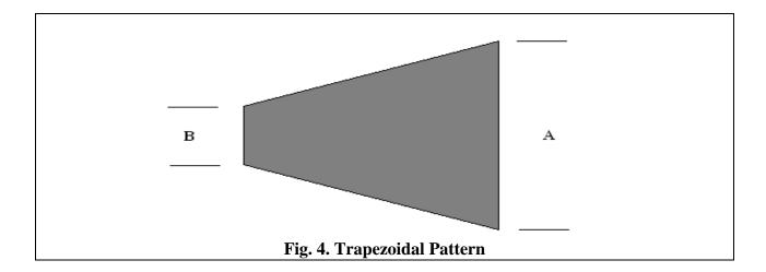
Use the definitions of the trapezoidal pattern and modulation index to show that the modulation index may be determined from the scope display<sup>2</sup> by:  $a = \frac{A - B}{A + B}$ .
