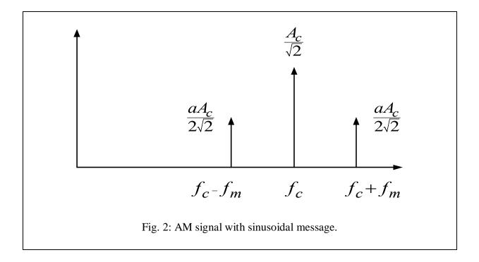
If the message is a tone, the AM signal will be as shown in Figure 2. (RMS values are shown in Figure 2; hence the factor of  $\sqrt{2}$ .) Furthermore, the spectrum analyzer provides no phase information (it is a scalar radio receiver); it displays the one-sided spectrum. On the other hand, a -Vector Signal Analyzerøis capable of processing phase information and is frequently used to analyze digitally modulated signals.
