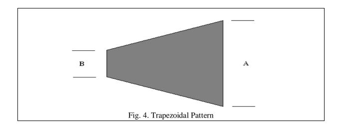
Use the definitions of the trapezoidal pattern and modulation index to show that the modulation index may be determined from the scope display<sup>2</sup> by:  $a = \frac{A - B}{A + B}$ .
