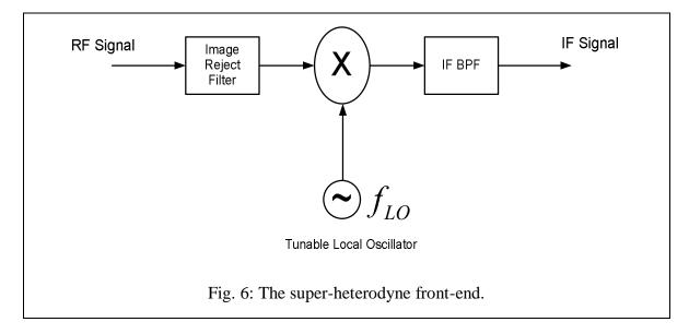
A simple super-heterodyne front-end consists of:
