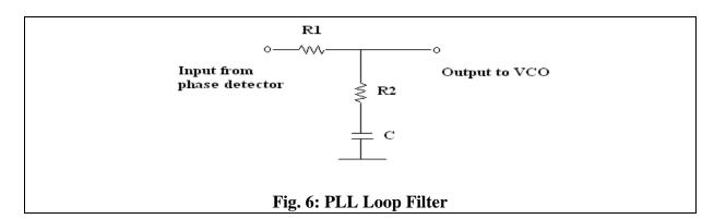
**7a.** The damping factor  $\zeta$  can be adjusted by the 1 k $\Omega$  pot, (R2), shown in Figure 5. Adjust R2 to observe the effects of changing the damping factor. You should see waveforms similar to those shown in Figure 7a, b, c, and d, below.
