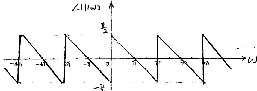
2. (25 pts.) The signal  $x[n] = \cos(2\pi n/3)$  is input to a digital filter with frequency response magnitude and phase as shown:
