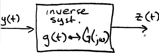
$$\begin{aligned} \frac{d^2 z}{dt^2} + 3 \frac{dz}{dt} + 2 z(t) \\ = \frac{d^2 y}{dt^2} + 6 \frac{dy}{dt} + 9 y(t) \end{aligned}$$
