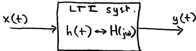
$$\frac{d^2y}{dt^2} + 6 \frac{dy}{dt} + 9y(t) = \frac{d^2x}{dt^2} + 3 \frac{dx}{dt} + 2x(t)$$
