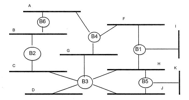
Consider the network above. Assume that the spanning tree algorithm is used. Assume that B1 has a lower id than B2, which has a lower id than B3, and so on.
