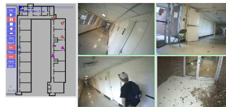
Figure 3. Visualization of video streams recorded by stationary (orange circular sectors) and moving (green circles) cameras. A moving camera is outfitted on the head of an moving agent. Selected agents are showing in magent color.
