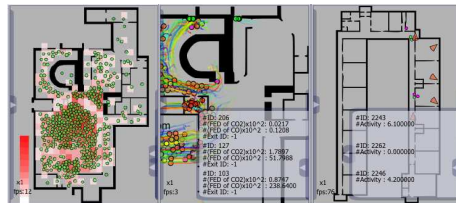
Figure 1. Visualization of Personnel-related information: (Left) congestion visualization, (Middle, Right) visualization of individual information (health level, activity level), and (Middle) visualization of current position and path of personnel.
