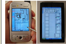
Figure 5. Our mobile visual analytic system running on mobile devices: (Left) Sprint PCS Vision SM smart device PPC-6700, and (Right) OQO 02.
