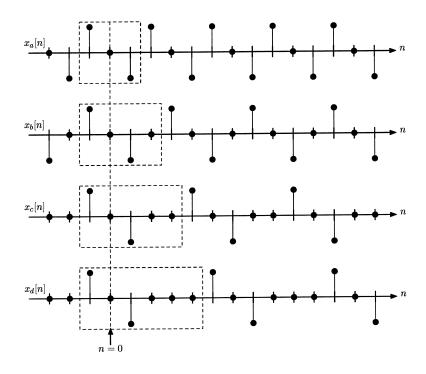
**Problem 3.** Using the DTFT to simplify computation of DTFS. [40 pts. total, **LO-iv**] Four periodic signals are given in the drawing above. All are created from an elementary signal  $x[n] \stackrel{\text{def}}{=} \delta[n+1] - \delta[n-1]$  by repeating it periodically. For example:
