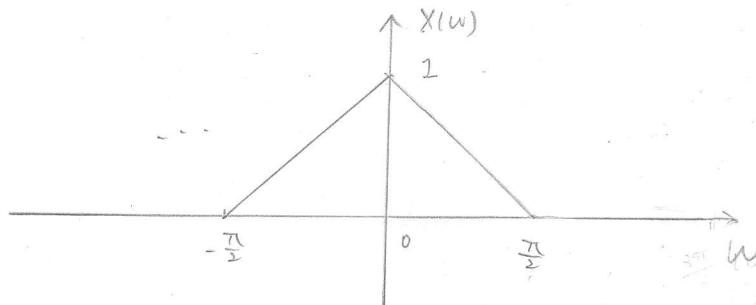
b.  $y[n] = x[Dn] \longleftrightarrow Y(w) = \frac{1}{D} \sum_{k=0}^{D-1} X\left(\frac{w-2\pi k}{D}\right)$
