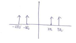
(10 pts) b) Suppose the signal x(t) is modulated by the carrier signal c(t) = $e^{10j\pi t}$ . Sketch the graph of the modulated signal in the frequency domain.
