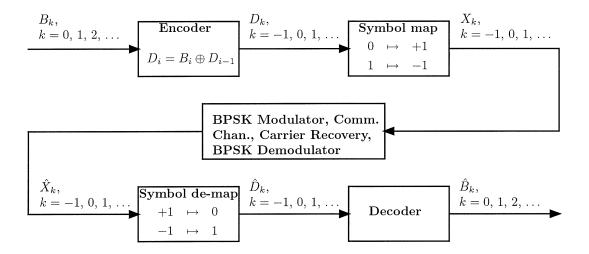
**Problem 1.** [25 pts. total] Consider the differentially encoded BPSK system described on the previous page focusing on the Encoder and Decoder blocks.
