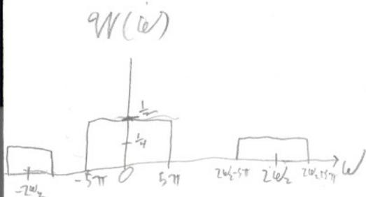
3 You then apply a lowpass filter with gain 2 to  $w(t)$ , making sure the cutoff  $\omega_c$  is such that  $5\pi < \omega_c < 2\omega_c - 5\pi$ . The lowpass filter output is  $x(t)$ .
