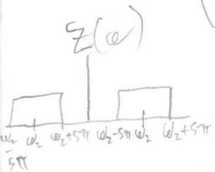
Yes. Since  $\cos(\omega_2 t) = \frac{1}{2}(e^{j\omega_2 t} + e^{-j\omega_2 t})$ ,  $z(t) = x(t)\cos(\omega_2 t)$  produces two copies of  $X(\omega)$  at  $+\omega_2$  and  $-\omega_2$ .  $Z(\omega) = \frac{1}{2}(X(\omega - \omega_2) + X(\omega + \omega_2))$  by (12). The Nyquist rate is then  $\omega_N = 2(\omega_2 + 5\pi)$  as can be seen in the figure at left.
