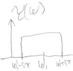
Yes. By (12),  $Y(\omega) = X(\omega - \omega_1)$ . This is the same as  $X(\omega)$ , recentered on  $\omega_1$  (see figure at left). The maximum frequency magnitude is then  $|\omega_1| + 5\pi = \omega_N$ . The Nyquist rate  $\omega_N = 2\omega_M = 2\omega_1 + 10\pi$
