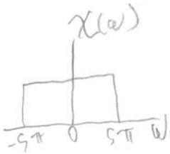
Yes.  $X(\omega) = u(\omega + 5\pi) - u(\omega - 5\pi)$ , which is 0 for  $|\omega| > 5\pi$ . Thus, the Nyquist rate is  $2 \cdot 5\pi = 10\pi = \omega_N$  by (19)
