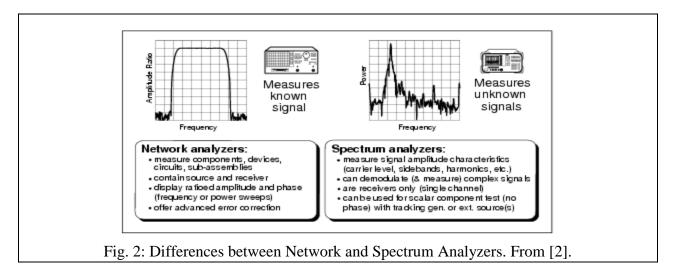
Roughly speaking, in addition to the forward gain, you also need to know the input resistance, the output resistance, and the reverse gain to characterize a two-port. And all of these can be functions of frequency. Vector network analyzers determine both the amplitude and the phase associated with these functions of frequency. Scalar network analyzers determine only the amplitude.
