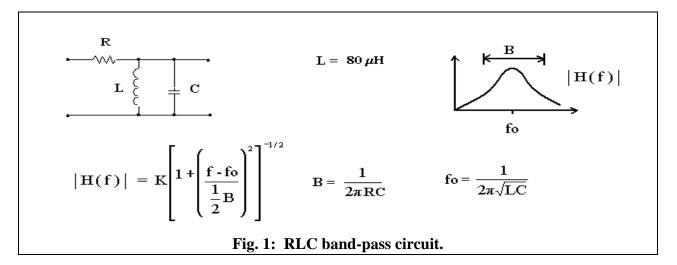
Select C for fo = 400-500 kHz. Select R so that the 3-dB bandwidth, B, is 100 kHz. Determine the step response of this circuit (hint: a step input can be simulated through the use of a sufficiently low-frequency square wave) observe the output of the system using an **oscilloscope**.
