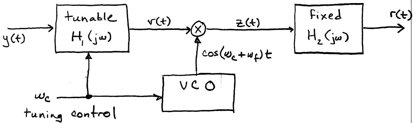
Goal is to analyze this superheterodyne receiver for the filter shapes given.
