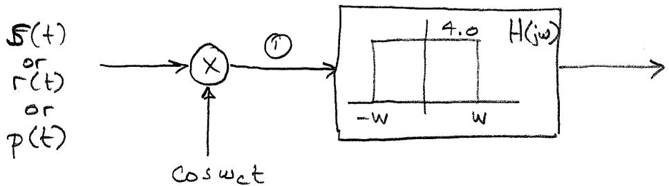
works as a demodulator for any of the signals as longs as  $w = w_c$  (and Tx, Rx oscillators in-phase)
