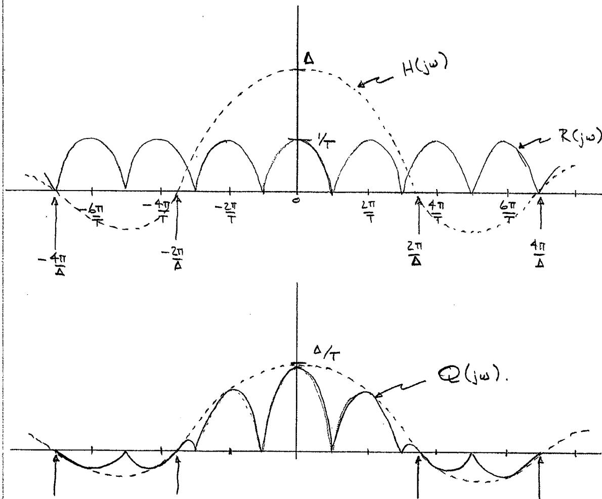
Picture Drawn for case where 1st zero crossing of sinc is past the band edge of 1st replication of  $X$  spectrum ie
