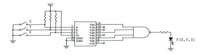
Determine the **ON set** and a simplified **minimum sum-of-products** function realized by this decoder-based circuit.
