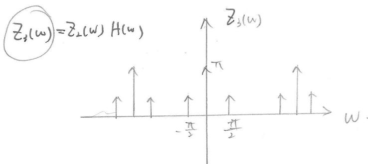
$$\begin{aligned} Z_3(\omega=0) &= \pi \tilde{d}(0) \\ Z_3(\omega=\frac{\pi}{2}) &= 2\tilde{d}\left(\frac{\pi}{2}\right) = \frac{1}{2} = \tilde{d}(0) \end{aligned}$$
