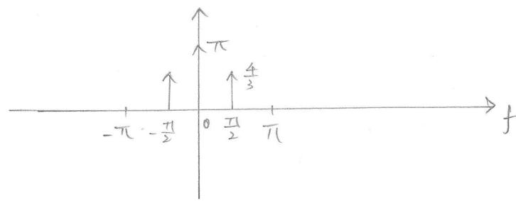
$$Z_3(\omega = \frac{\pi}{2}) = \frac{1}{T_s} \frac{1}{\pi} (2\pi T_s) d(\omega - \frac{\pi}{2})$$
